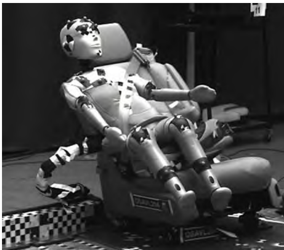
Test images of the LODC on a 45 degree reclined seatback angle during a lateral oblique impact before the LODC reached maximum head excursion: with the booster seat (left) and without the booster seat (right).
