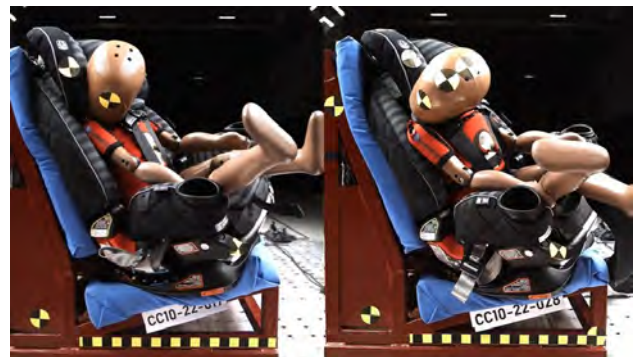
Head rotation and roll-out observed in far-side impacts for the tight harness (left) and loose harness (right) conditions.
