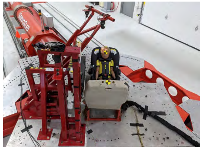
A Q1.5 ATD seated in a rearward-facing infant CRS with a support leg attached with rigid lower anchors to the test bench with a door surrogate. The test buck is rotated 30° relative to the test sled.
