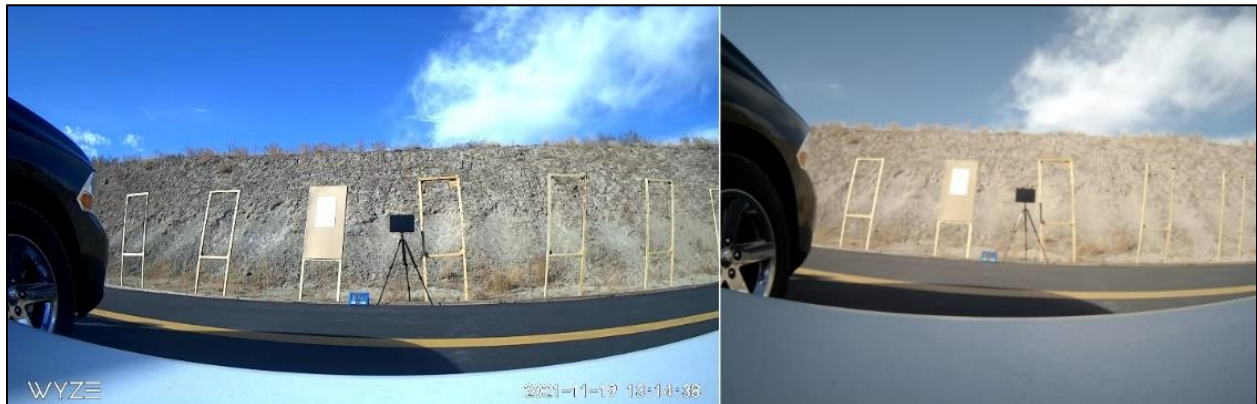
Figure 17 – Two different security cameras capture varying color at the same time
