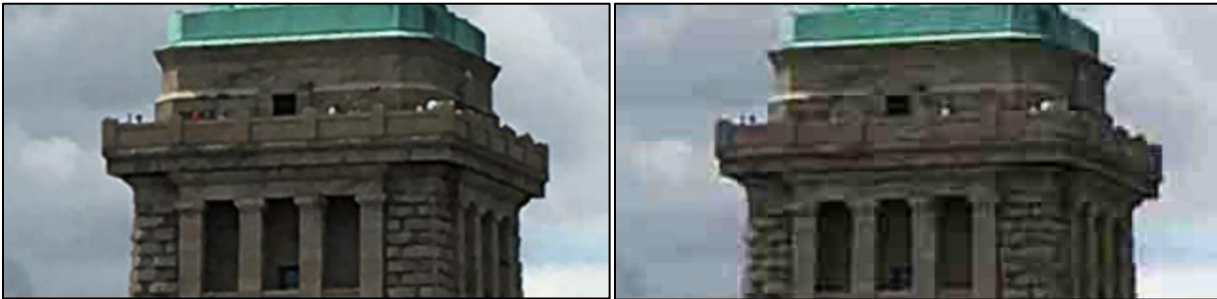
Figure 12. Uncompressed image (left) and same image compressed (right) with the artifacts
