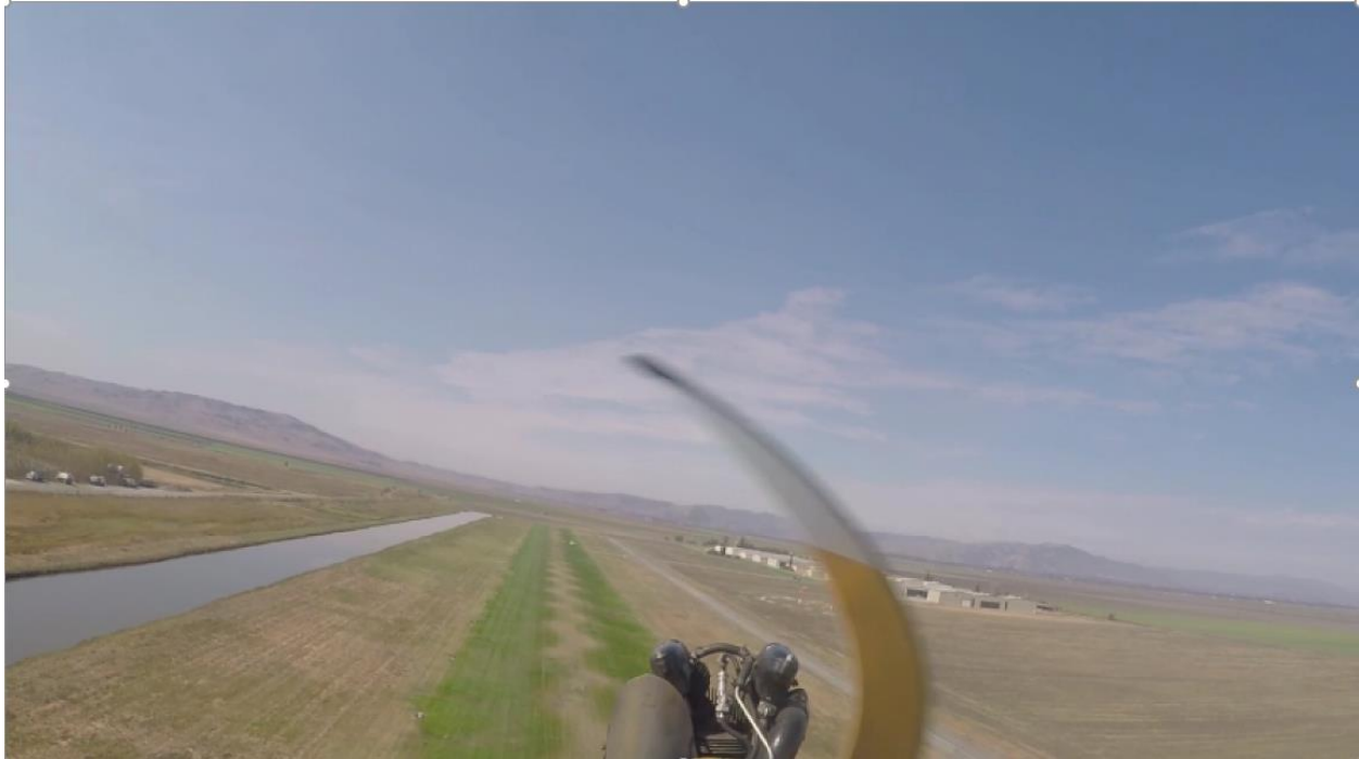
Figure 22 – Sample of rolling shutter, straight objects may appear curved
