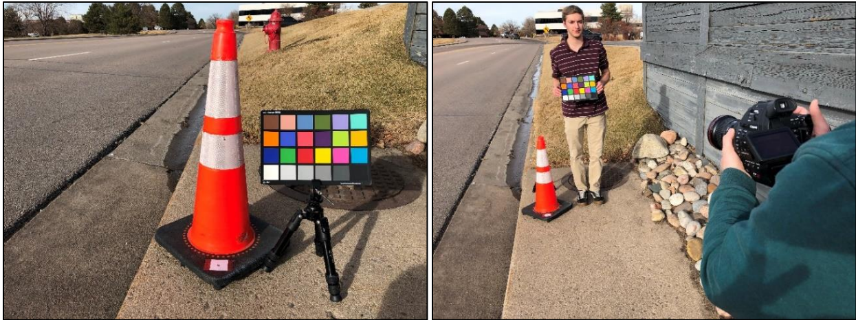
Figure 27 – Color Correction Chart used to calibrate digital images
