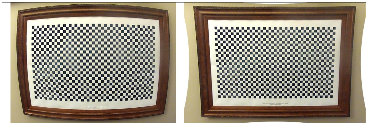
Figure 16 – Comparison of an image without correction (left) and corrected (right)
