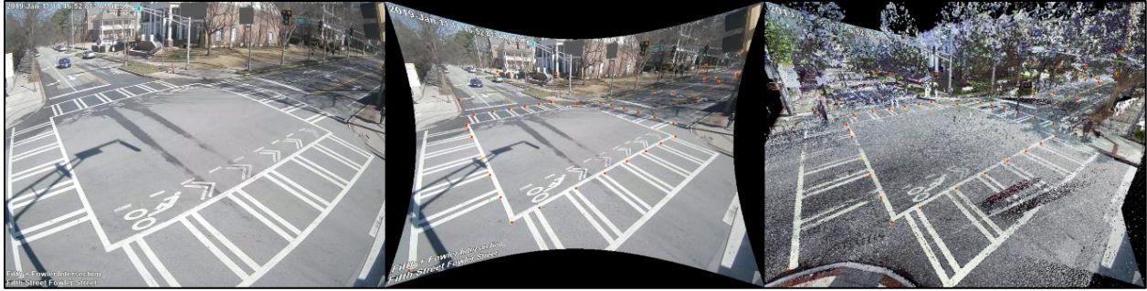
Figure 6: Original merged frame (left), lens distortion corrected frame (middle), and three-dimensional scan data overlaid on lens distortion corrected frame (right).
