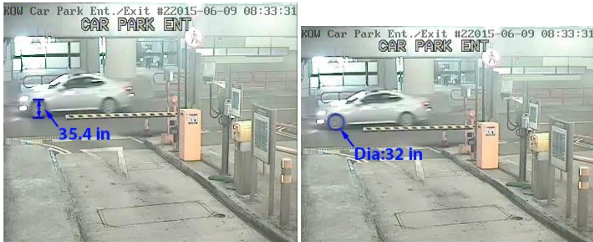
Figure 15 – square PAR stretched vertically (left), .9 PAR corrected so objects appear unstretched (right)
